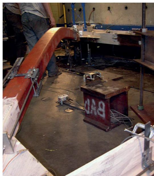
Figure 1. Inelastic brace buckling failure [1]
