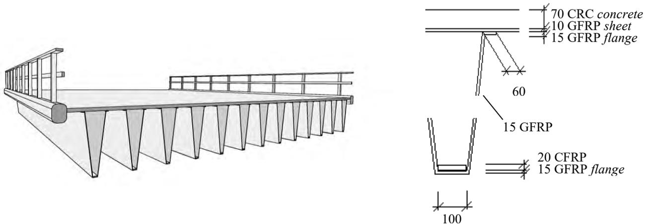
Fig. 1: Outline of the *i-bridge* concept, a perspective sketch illustrating the major components of the bridge and to the right some details of the deck and the bottom of the beams (dimensions in mm).
