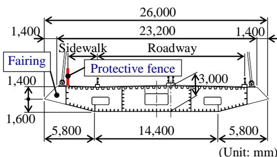
Fig. 2: Detail of stiffening girder (planned)
