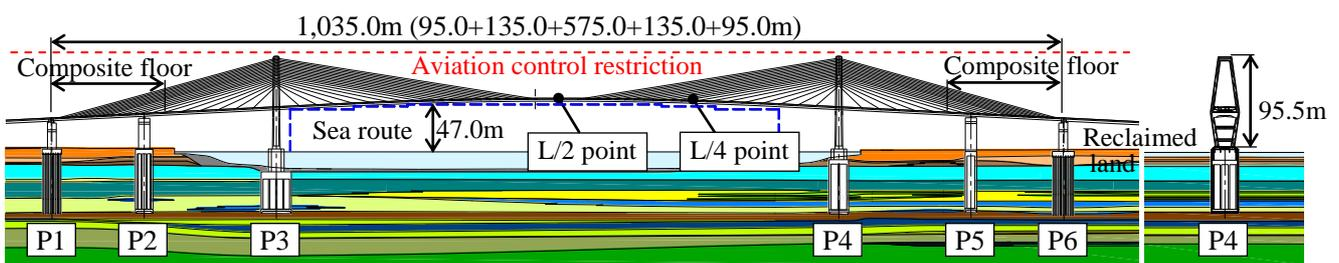
Fig. 1: General view of cable-stayed Bridge (planned)
