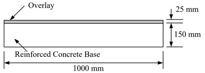
Fig. 1: Overlay Specimen Details
